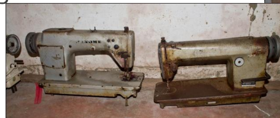
Nine (9) units high speed sewing machine, all damaged by sea-water
